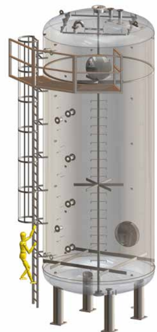
▲ Figure 1: Overview of the 90-m 3 ice slurry storage unit.
