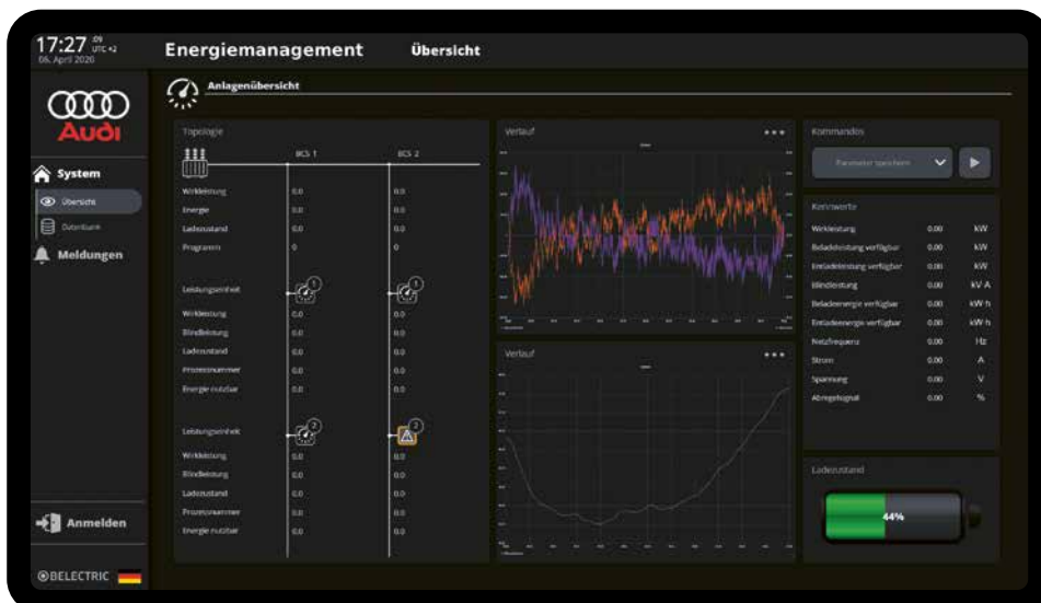
▼ User interface of the energy management system for data display and management of a battery storage power plant.
